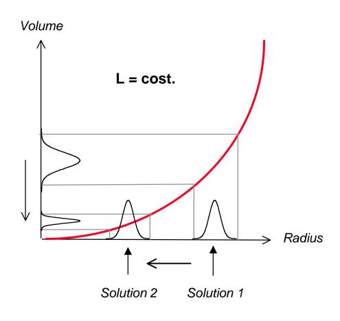
Robustness achieved in solution 2 (compared to solution 1) is due to the non linear relationship between 'radius' and 'volume'.
