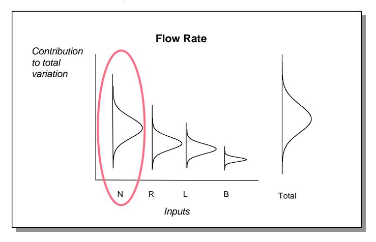
The next step would be to tighten tolerances. This generally requires using more expensive components and processes.
