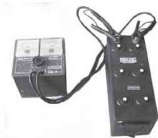
Figure 8: Carbon pile load tester
