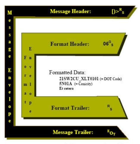
Complete message:  $D^R_{g}06^G_{g}21SW2CU\_XLT0101^G_{g}5N01A^R_{g}O_{T}$
