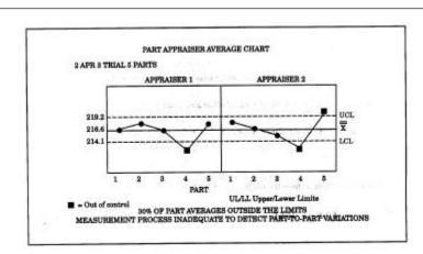
There are three points that fall outside the limits and so the measurement process is not adequate to detect part-to-part variations.
