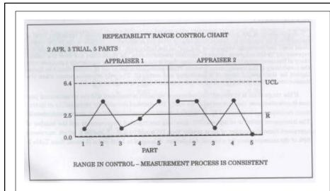
All the points are within limits( $UCL_R$  and  $LCL_R$ ) and so the measurement process is under control and is said to be consistent.
