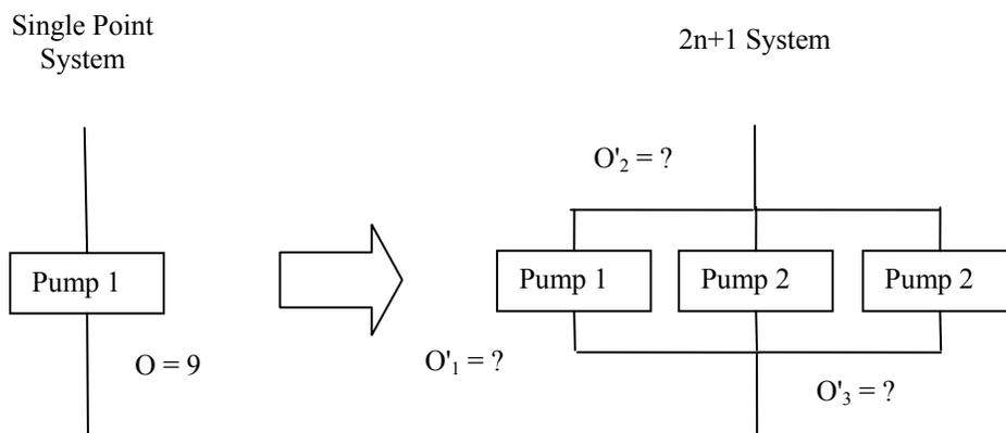
Figure 4-6. Single point system vs. redundant system
