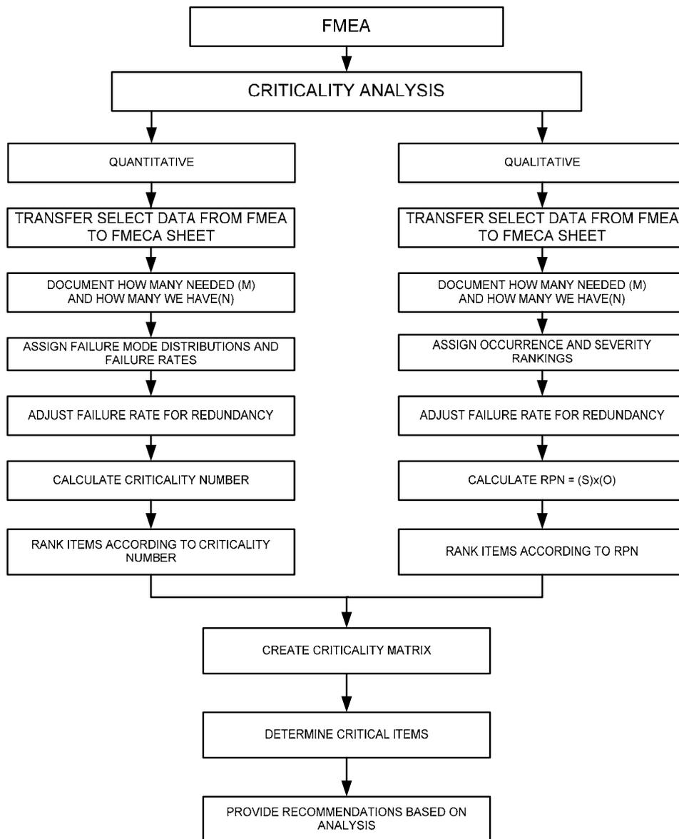
*Figure 4-1. FMECA flow*
